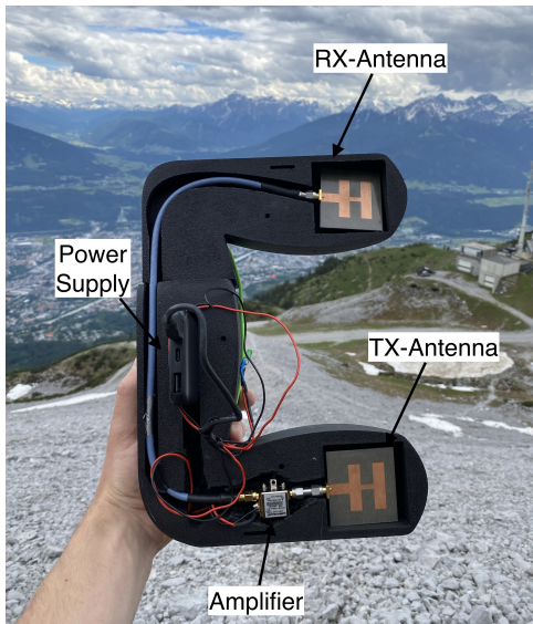
Fig. 3: The assembled AT in the designed cover for protection
